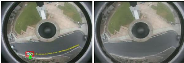
Figure 7: Tracking of a vehicle in omni video sequence. Bounding box is shown in red, with track id in green, and the track history as a yellow line. Image on right shows the current estimate of the background image. Note that the moving vehicle has got removed in the background image.
