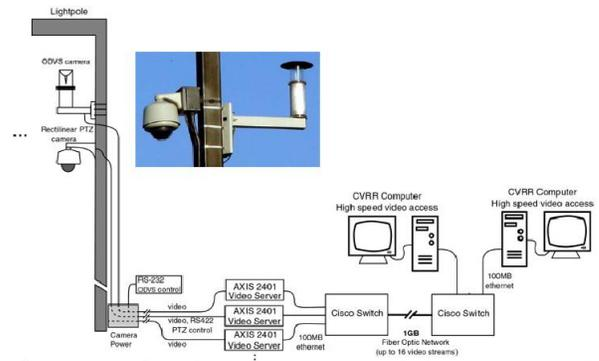
**Figure 6: Outdoor Video Clusters provide continuous streaming video of roads and other areas over standard or high-speed networks.**
