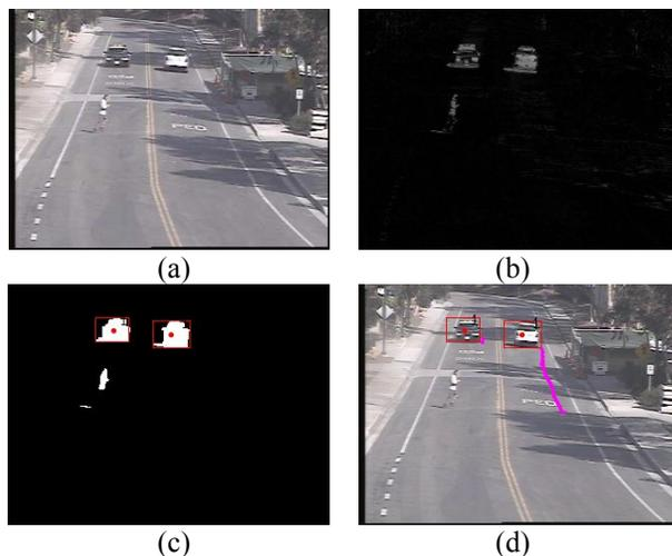
**Figure 3 Steps in the implementation of vehicle tracking algorithm: (a) Original frame from the video sequence (b) Output after background subtraction (c) Identification of vehicle regions (d) Tracking over frames using Kalman filter.**
