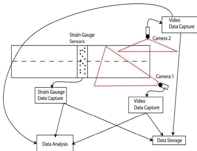
**Figure 8 Block diagram of seismic and video event capture system**
