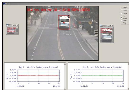
**Figure 4 Snapshot of the vehicle detection and tracking application. The detected vehicles in left and right lanes are identified and snapshots of them shown on the side are archived. The bottom figures show the output from the strain gauge sensors. Note that the current implementation**
