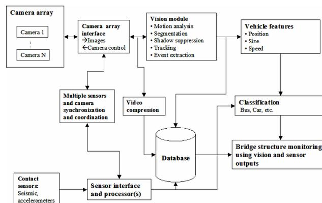
**Figure 1** Block diagram for structural health monitoring of bridges
