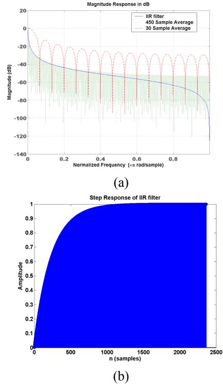
**Figure 2 (a) Magnitude response of IIR low-pass filter in frequency domain (b) Step response of IIR low-pass filter in time domain.**
