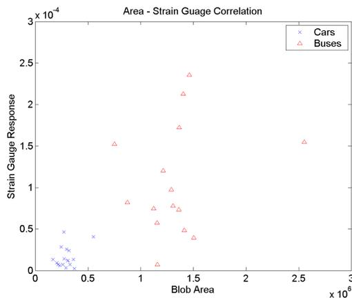
**Figure 11 Scatter plot of data associated with each vehicle. X-axis corresponds to the blob area, and Y-axis corresponds to the strain gauge response. Two clusters corresponding to cars and buses (verified ground truth) can be distinguished.**
