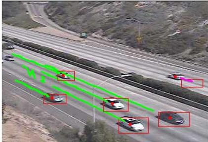
**Figure 5 Results of vehicle detection and tracking algorithm on freeway traffic.**
