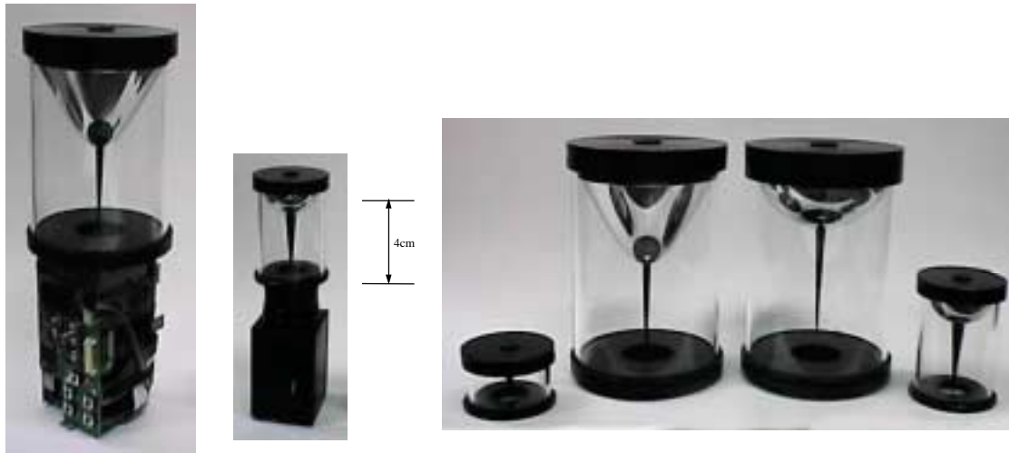
(a) C-ODVS with a hyperboloidal mirror (b) Ultra C-ODVS with a spherical mirror
