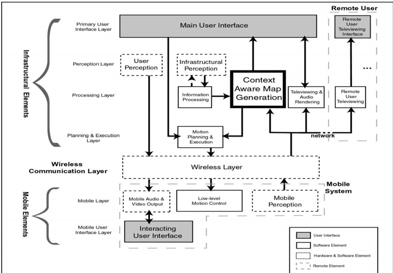
**Figure 1: The system architecture has distributed sensing and processing elements and uses the context aware map to maintain and display information to the user**
