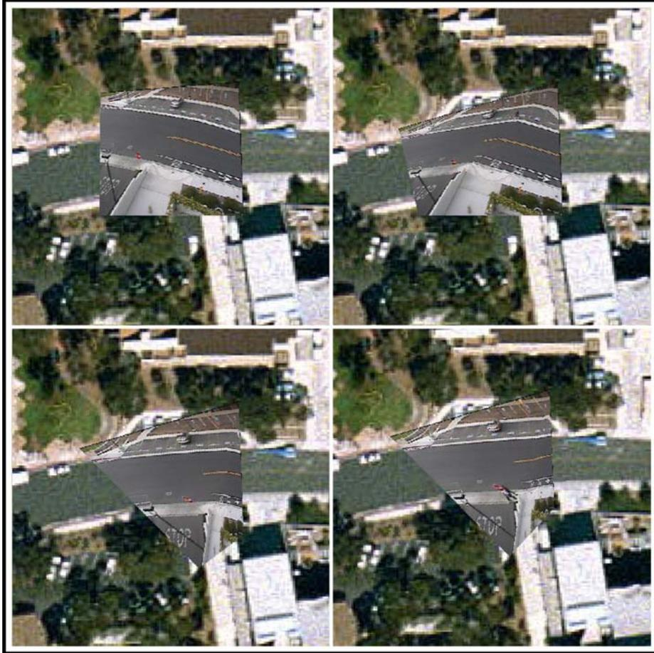
**Figure 6: Live video overlay is accomplished using a 4-point registration process and aligning the road correctly with the background**
