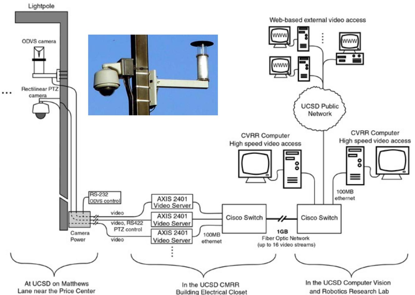
**Figure 3: Outdoor Video Clusters provide continuous streaming video of roads and other areas over standard or high-speed networks**
