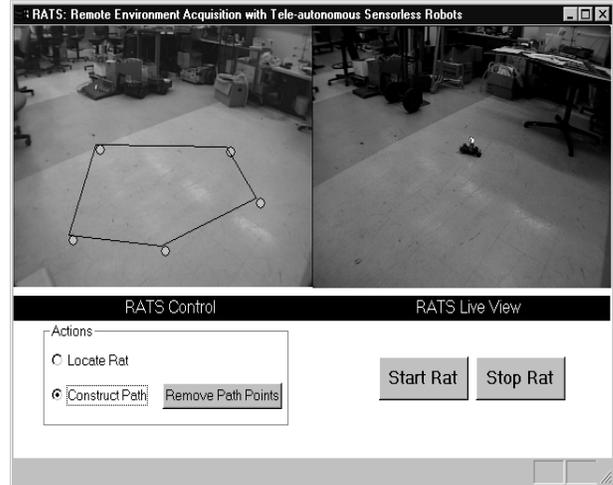
**Figure 6. Web-based teleautonomous operation of a mobile probe. The user specifies only the path which the remote probe traverses autonomously.**
