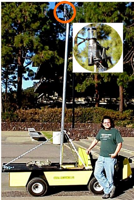
**Figure 3. Mobile unit for video capture and communication is used for acquiring traffic data**
