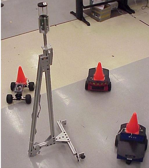
**Figure 7. Multiple mobile units and ODVS during experimental trials.**
