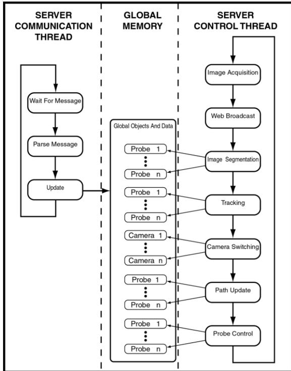
**Figure 5. Overview of the server side software for realizing web-based teleautonomy of the mobile video probes.**
