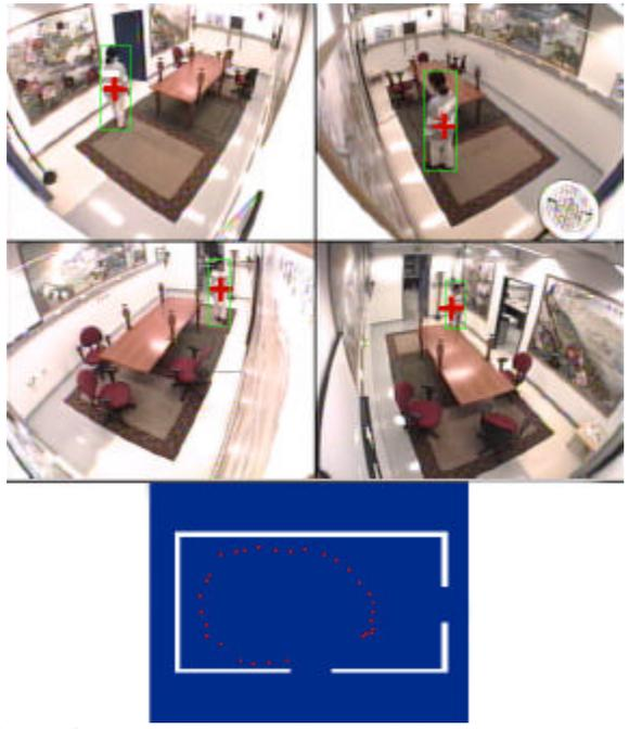
**Figure 3.** 3D tracking – smaller crosshairs (barely visible) and green bounding boxes are segmentation results used by the tracker to compute 3D tracks and bounding cylinders. Larger crosshairs are projections of tracks back onto the image planes. Bottom: projections of the track onto the floor plane.
