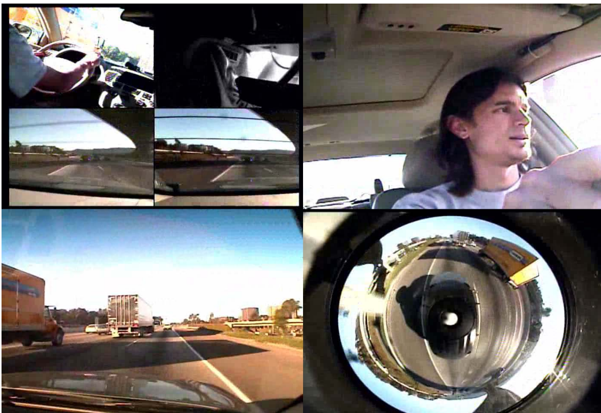
Figure 11: LISAQ collects video from 8 different cameras which capture the interior and surround of the vehicle.
