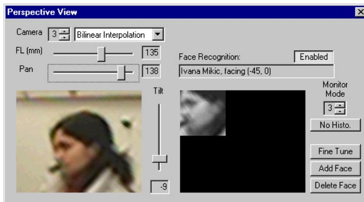
Figure 4: Face perspective view generation and face recognition.
