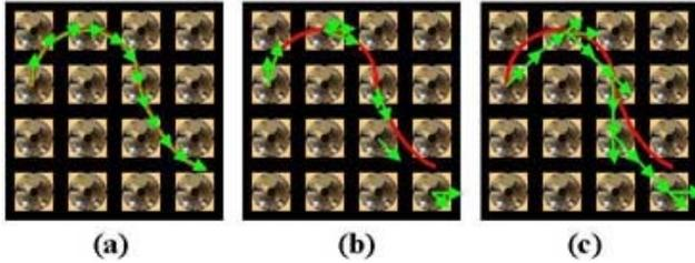
Figure 4: (a) Desired, smooth walk path for view synthesis. (b) Discrete paths with camera switching to approximate the desired path. (c) Discrete interpolation between camera pair with zooming stereo.
