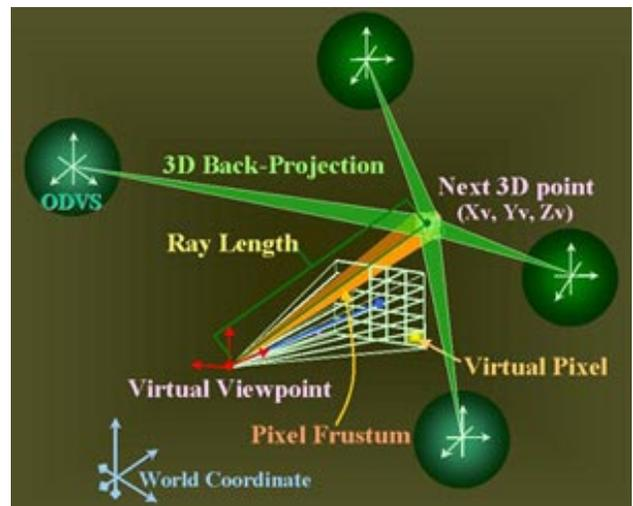
Figure 5: Multiple camera stereo with range-space search.
