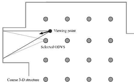
**Figure 6:** Plenoptic representation based on coarse structure of the environment.
