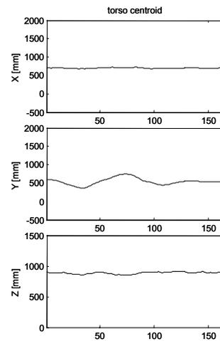
Figure 7 Torso centroid as a function of time for the sequence containing a sitting person
