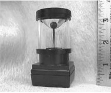
Fig. 1. Compact and low-cost ODVS
