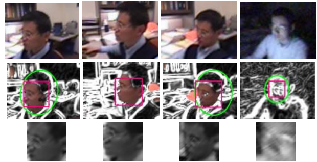
Figure 5: Some results of the multi-primitive face detection and tracking. Top row shows various backgrounds and lightings, middle row shows combined skin-color and edge detections, and lower row shows the cropped faces.
