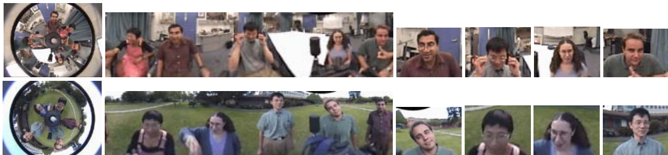
Figure 8: Sample indoor and outdoor images from the test and training video sequences for face detection, tracking, and face orientation estimation. Left to right: the source omni-videos, the unwarped panoramas, and human perspectives.
