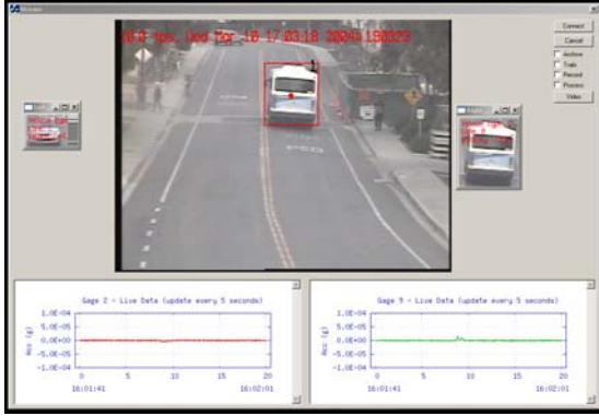
Figure 7 Snapshot of the vehicle detection and tracking application. The detected vehicles in left and right lanes are identified and snapshots of them shown on the side are archived. The bottom figures show the output from the strain gauge sensors. Note that the current implementation has a delay in getting sensor output, hence the blip due to the vehicle is not visible in the image.
