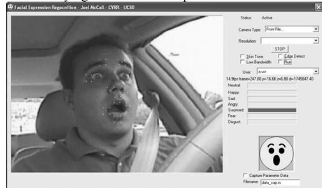
Figure 7 Driver State Analysis in the LISA-Q test bed
