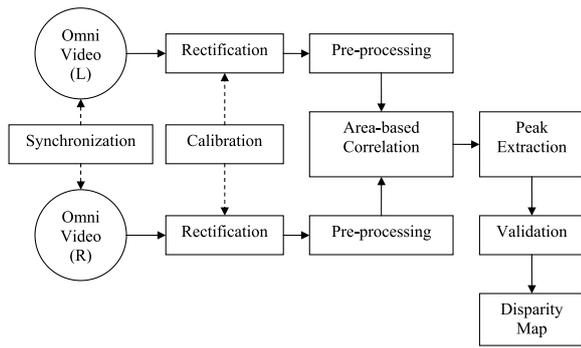
**Fig. 1.** Block diagram of stereo analysis from vehicle mounted omni cameras.
