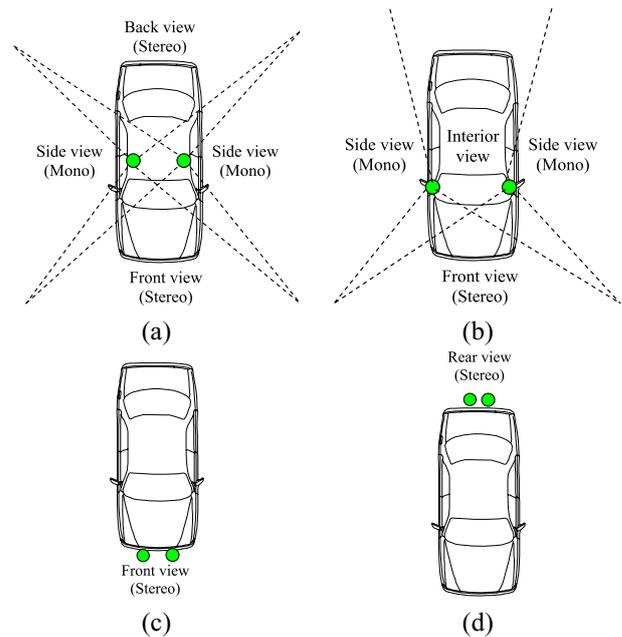
**Fig. 2.** Omni-camera configurations for stereo analysis with cameras mounted on (a) Top (b) Sides (c) Front (d) Rear of the automobile.
