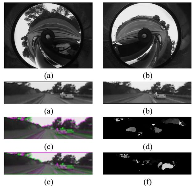
**Fig. 3.** Rectified perspective virtual views generated from the two omni cameras. The epipolar lines are along the rows of both the cameras. (c) Combined image. Note that due to calibration errors, there is some vertical displacement between features. (d) Depth map obtained using SRI SVS software. (e) Combined image after correcting the vertical disparity (f) Depth map obtained after correction.
