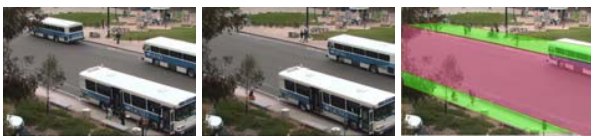
Figure 11: Example frames contained in multiple backgrounds for bus station and site modeling; red and green regions represent watch zone and pedestrian zones, respectively.
