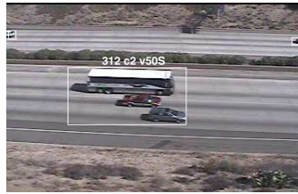
(b) Vehicle 312: Tracking error combines bus with other vehicles
