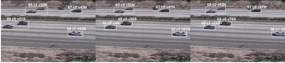
(d) Vehicle 68,69: Track classification quickly recovers after tracking error
