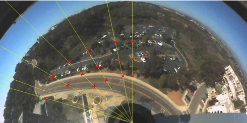
Fig. 2. Calibration correspondence points. Yellow rays represent changes in pan position and red points represent tilt positions for that pan value.
