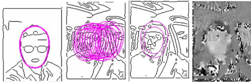
Fig. 7. Head detection process: the initial ellipse on thermal edge map, ellipse search on color video's edge map, a fitted ellipse, and skin likelihood, respectively.
