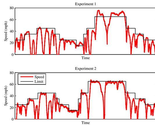
**Fig. 4. Results of sample Test Run for Experiment 1 - No Display (top) and Experiment 2 - Warning sign (bottom). The driver's ability to maintain speed is evidenced clearly by the reduced amount of time accidentally spent over the speed limit in Experiment 2.**
