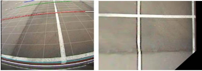
Fig. 4. Illustration of ground-grid alignment in the ground-truth camera, and the resulting flat-plane transformed image. Radial distortion is taken into account as can be seen by the bowed lines.
