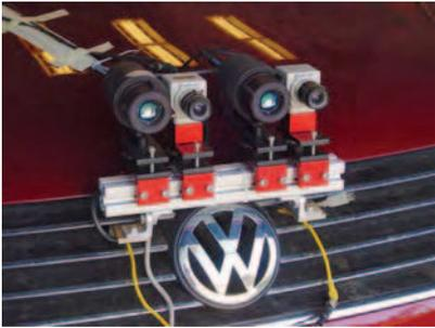
Fig. 9. Experimental testbed: Two color cameras and two infrared cameras arranged in stereo pairs and mounted to the front of the LISA-P testbed.
