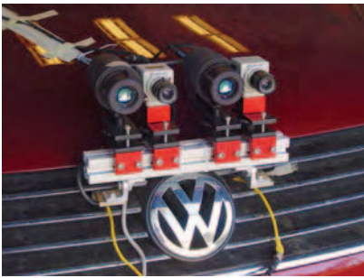
Fig. 9. Experimental testbed: Two color cameras and two infrared cameras arranged in stereo pairs and mounted to the front of the LISA-P testbed.
