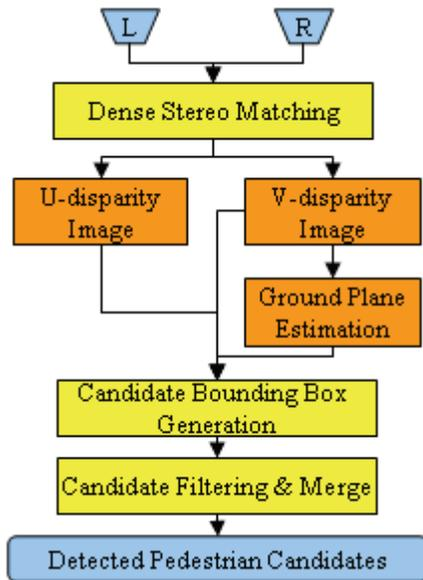
Fig. 1. Flowchart of stereo disparity-based obstacle detection algorithm.
