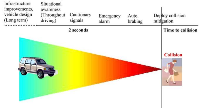
Fig. 1. Timeline of pedestrian protection measures (based on the study in [44]). The reaction time for a given distance decreases with vehicle speed.
