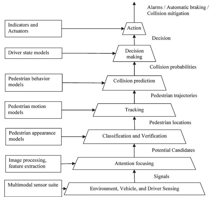
Fig. 2. Vehicle and infrastructure-based pedestrian detection. Data flow diagram showing distillation of information from raw signals up to appropriate action.
