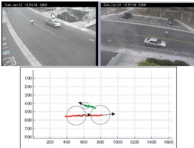
Fig. 6. Estimation of interaction patterns of moving objects with different velocities using the homography-mapped footage regions in the projection planes. Green track corresponds to the walking person, and red track corresponds to the car [75].
