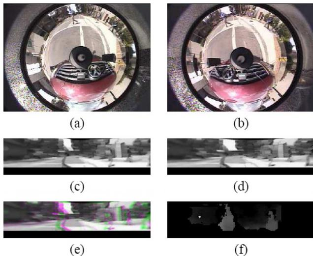
Fig. 4. (a) and (b) Images taken from stereo omniconic cameras in front of the vehicle. (c) and (d) Rectified perspective virtual views generated from the two omniconic cameras. The epipolar lines are along the rows of both the cameras. (e) Combined image. (f) Disparity map with pedestrians having large disparities [30].
