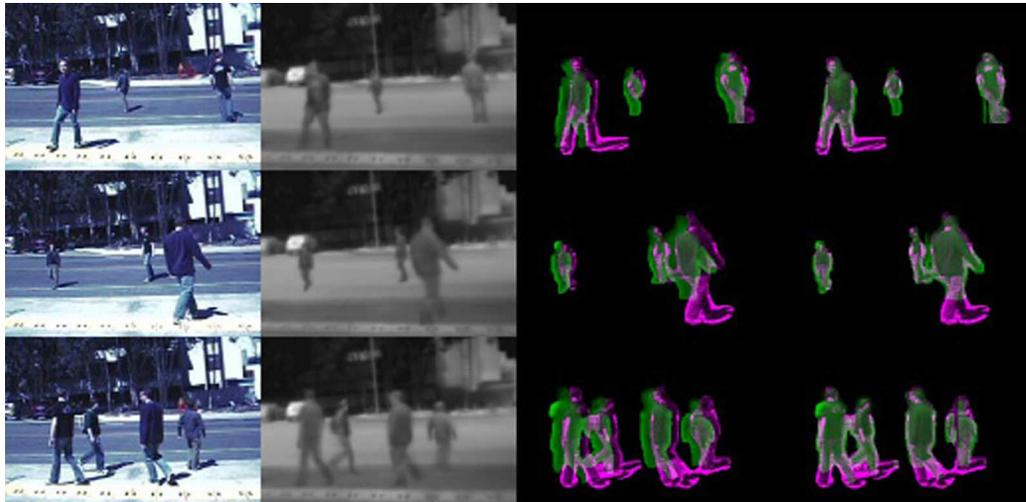
Fig. 5. Stereo registration between visible light and thermal images (a) input color image, (b) input thermal IR image, (c) unaligned overlay of color and IR foregrounds before registration, and (d) aligned overlay of color and IR foreground after registration [53].
