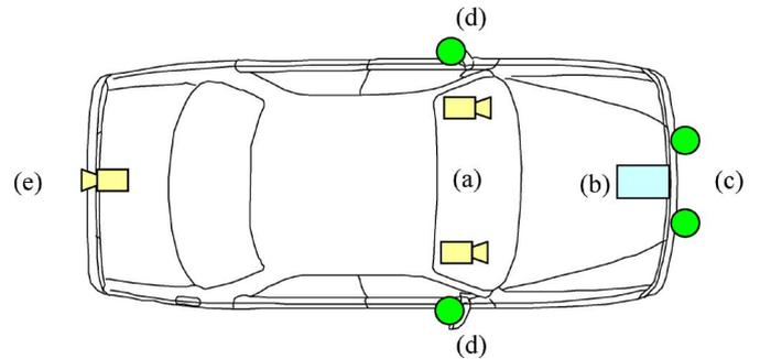
Fig. 3. Sensor configurations for detecting pedestrians and other objects. (a) Wide baseline stereo for distant objects. (b) RADAR for distance measurement in narrow FOV. (c) Narrow baseline wide FOV (omni) stereo pair for near objects. (d) Omnicameras to monitor blind spots. (e) Monocular reverse camera.
