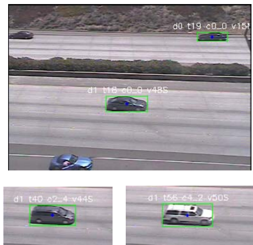
Fig. 3. Image and track based classification (a) cars (b) van (c) SUV. Note that (b) and (c) were misclassified using single image but correctly classified using full track [6].
