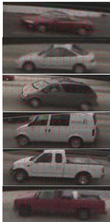
Fig. 4. Histogram of oriented gradients (HOG) representation of vehicle snapshots. The red arrows denote the gradient orientations with the length corresponding to the frequency of that orientation in the local histogram around that point.
