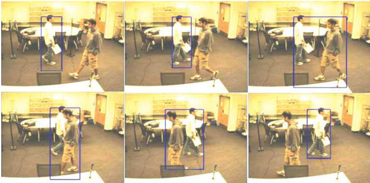
Figure 6. A successful tracking scenario where the track is maintained through merging, occlusion and divergence of foreground objects is shown here. By using the information from the other sensors through the iterative decoding scheme, the global tracker is able to maintain the track through an occlusion. Note that we are not using velocity constraints here and hence the global tracker has to rely on information from other sensors to maintain the tracks over such occlusions.
