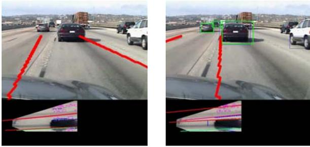
Fig. 6. a) Stand-Alone Lane Tracker Output, Frame 226. We note that although it is 0.133 seconds after the lane change, the lane tracker has not recognized the lane change yet, and indicates lane markers bisecting the vehicle in front. b) Lane and Vehicle Tracker has already changed lanes, as well as tracking the nearby vehicles.
