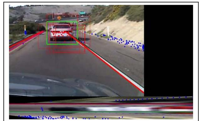
Fig. 5. Lane and Vehicle Tracking with candidate particles shown. Red boxes indicate a particle with medium confidence. Green boxes are the state predictions. Blue boxes are the vehicle detections. The bottom section shows a bird's eye view using the inverse perspective mapping.
