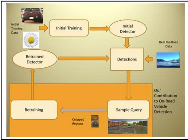
Fig. 4. Active Learning framework for on-road vehicle detection [22]
