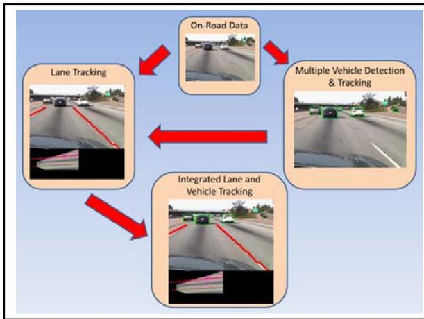
Fig. 2. Lane and Vehicle Tracking framework overview.
