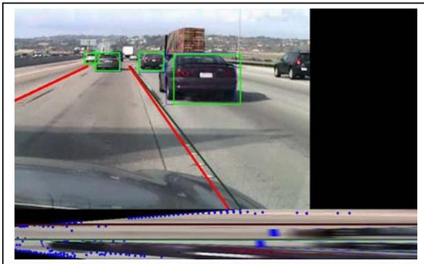
Fig. 7. Lane and Vehicle Tracking performance in dense traffic. The bottom section shows a bird's eye view using the perspective mapping.
