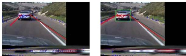
Fig. 11. a) Stand-Alone Lane Tracker Output, Frame 28. The blue circles indicate detected lane markings. We note that the lane tracker has picked up many erroneous lane markings due to the vehicle ahead, and as such, the tracked lanes are bisecting the vehicle. b) Lane and vehicle tracking. The lane markings that overlap with the tracked vehicle are ignored, indicated in red. The tracked lane markings are more accurate.
