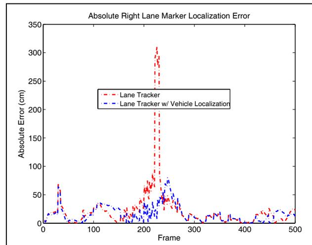
Fig. 9. Plot of absolute localization error vs. time, sequence 1. Note the spike in absolute error for the stand-alone lane tracker, as it does not detect the lane change until 9 frames after it has happened.
