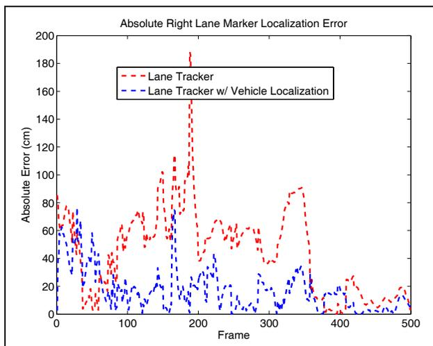
Fig. 10. Plot of absolute localization error vs. time, sequence 2. In this sequence, there are no lane changes, just lane following. Notice the error in lane tracking alone, caused by erroneous lane marker identification due to the vehicle ahead.
