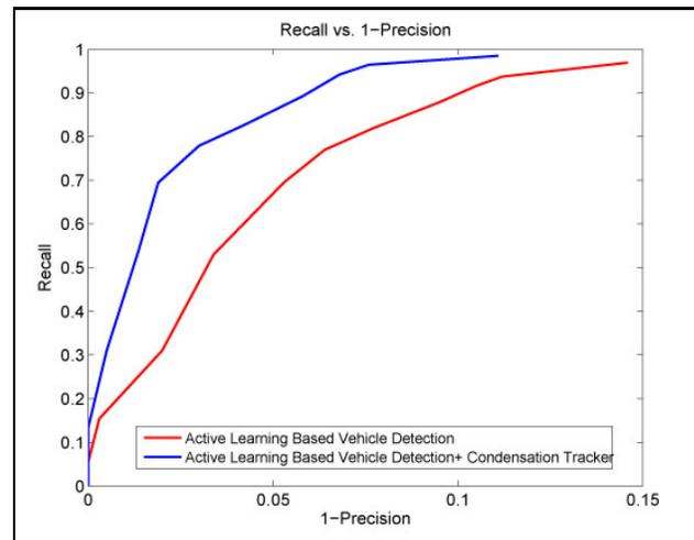
Fig. 8. Plot of *Recall vs. 1 - Precision* for active learning based vehicle detection, Sequence 1, and active learning based vehicle detection+condensation tracking. Note the improvement that tracking makes in system performance.
