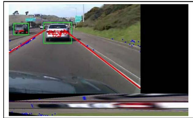
Fig. 1. Lane and Vehicle Tracking system performance. Green boxes indicate tracked vehicles, and red lines indicate tracked lane positions. Blue circles indicate markings used for lane localization. Red circles indicate lane markings that have been eliminated because of their overlap with tracked vehicles.
