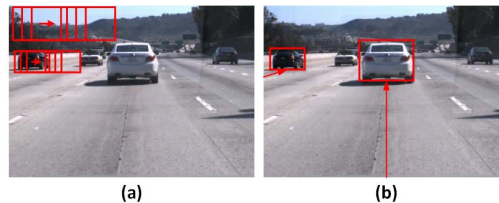
Figure 1. (a) Sliding window of multiple sizes used across the image, (b) Relationship between sliding window and the position of the leading vehicles.
