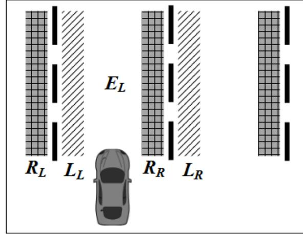
Figure 2. Definition of regions for lane drift detection
