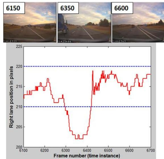
Figure 3. Sample result of the lane drift detection
