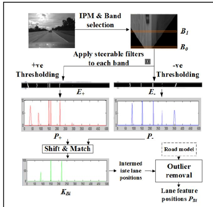
Figure 1 Efficient lane feature detection algorithm (LAsER).
