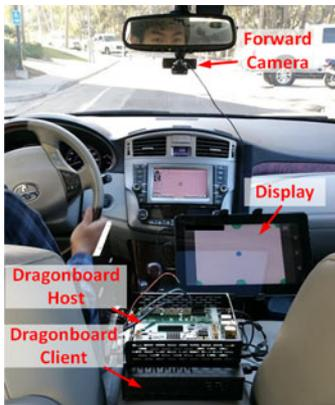
Fig. 6. Embedded system setup in our testbed with two Snapdragon 810 development boards that are connected to the cameras (rear camera is not seen in the image).
