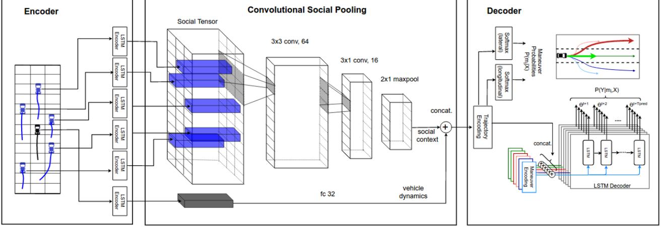
Figure 3. **Proposed Model:** The encoder is an LSTM with shared weights that learns vehicle dynamics based on track histories. The convolutional social pooling layers learn the spatial interdependencies of the tracks. Finally, the maneuver based decoder outputs a multi-modal predictive distribution for the future motion of the vehicle being predicted
