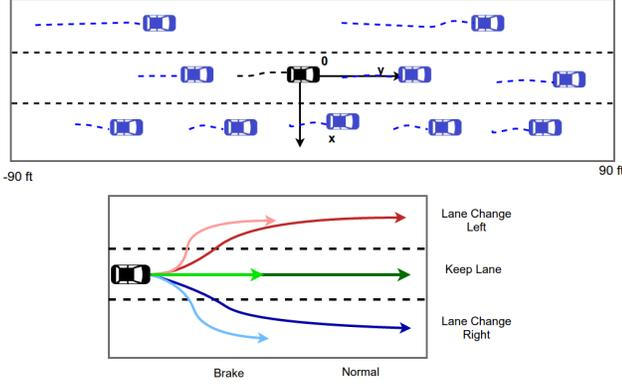
Figure 2. **Top:** The co-ordinate system used for trajectory prediction. The vehicle being predicted is shown in black, neighboring vehicles considered are shown in blue. **Bottom:** Lateral and longitudinal maneuver classes
