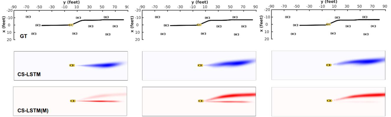
Figure 5. **Comparison of uni-modal and multi-modal predictions:** The figure shows the true trajectory (top, black), CS-LSTM predictive distributions (middle, blue) and CS-LSTM(M) predictive distributions (bottom, red) for three consecutive frames of a lane change maneuver. The heat maps are generated by plotting the Gaussian components for each maneuver at each time step in the prediction horizon
