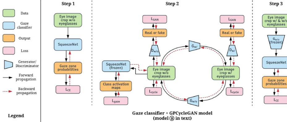
Fig. 4: Training setup and architectures for different gaze zone estimation models.
