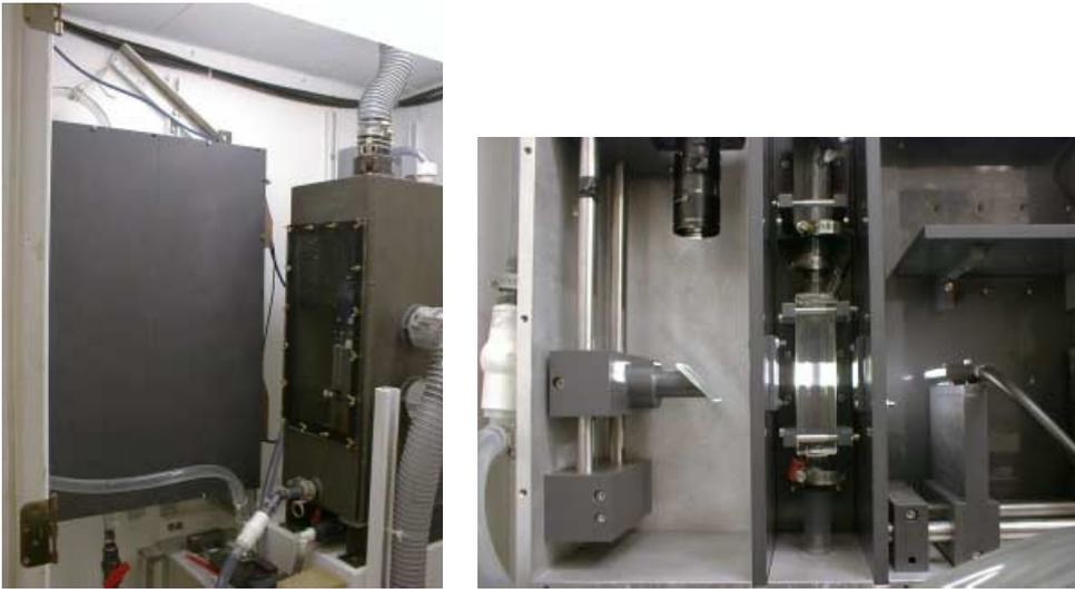
**Fig. 7a,b.** REFLICS flow-imaging module. **a** The housing (closed with gray PVC panels) mounted next to the CUFES's concentrator. **b** Inside of the housing, showing camera, flow tube, and illumination
