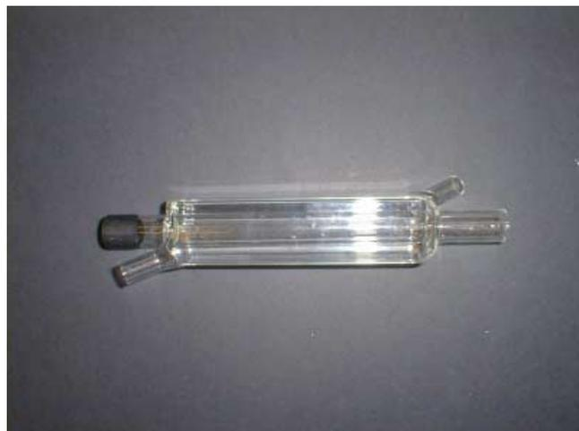
Fig. 6. Side view of REFLICS's glass flow cell. CUFES flow goes in and out from tubing protruding left and right. Water for the jacket flows in and out from smaller tubing protruding diagonally
