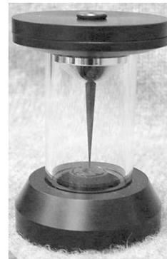
Figure 1. Compact omnidirectional vision sensor
