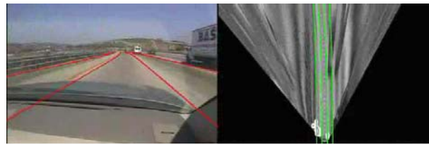
Figure 3. Lane tracking results overlaid onto video, aerial photograph of the road, and an inverse perspective warping of video.
