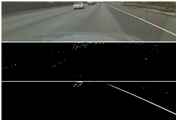
Figure 2. A typical highway scene in California (top), response for circular reflectors (middle), and response for solid line markings (bottom).
